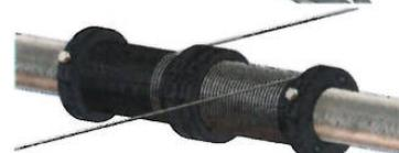
The newly developed cable drum has a helical groove in which the pull wire is fed in and rolled out. Because of this guide the wire makes no lateral contact, retains its original shape and is always in the right place, resulting in virtually no wear.
